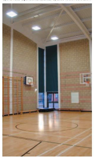
Natural light should be introduced into the gymnasium where possible. Blinds may be required to control glare and to provide privacy when required. Blinds should be incorporated within the cavity of the glazing units in the windows/screens.
